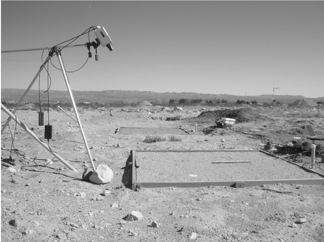
Fig 6. Picture of the FLIR thermal infrared camera at the New Mexico Tech land mine detection test facility.
