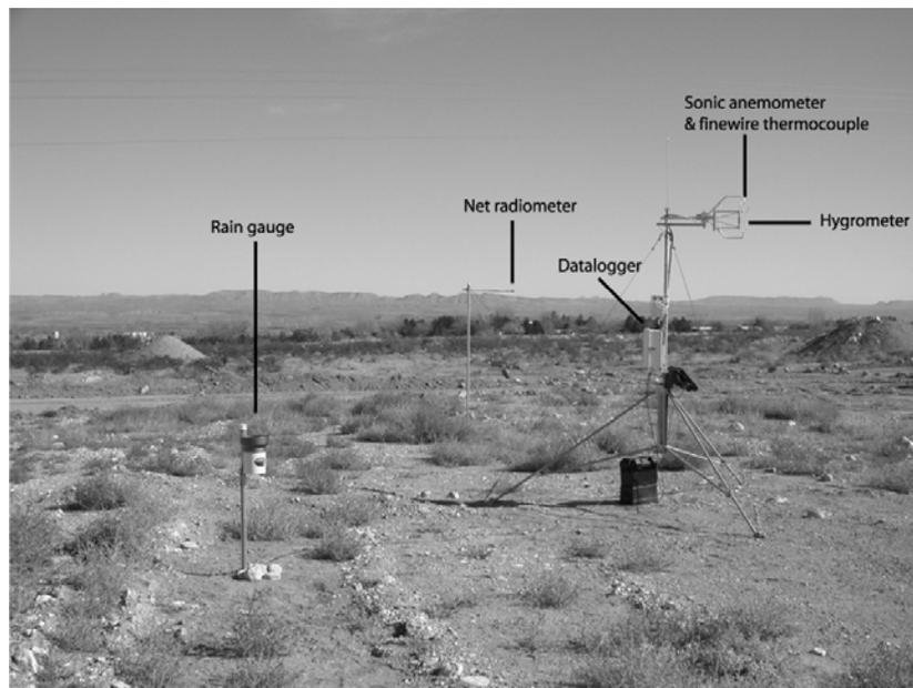
Fig. 4. Picture of the weather station.
