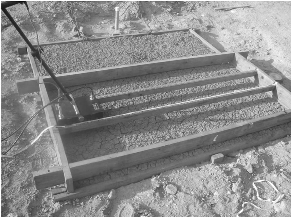
Fig. 6. Picture of pulseEKKO 900 MHz ground penetrating radar antennae and mounting frame.
