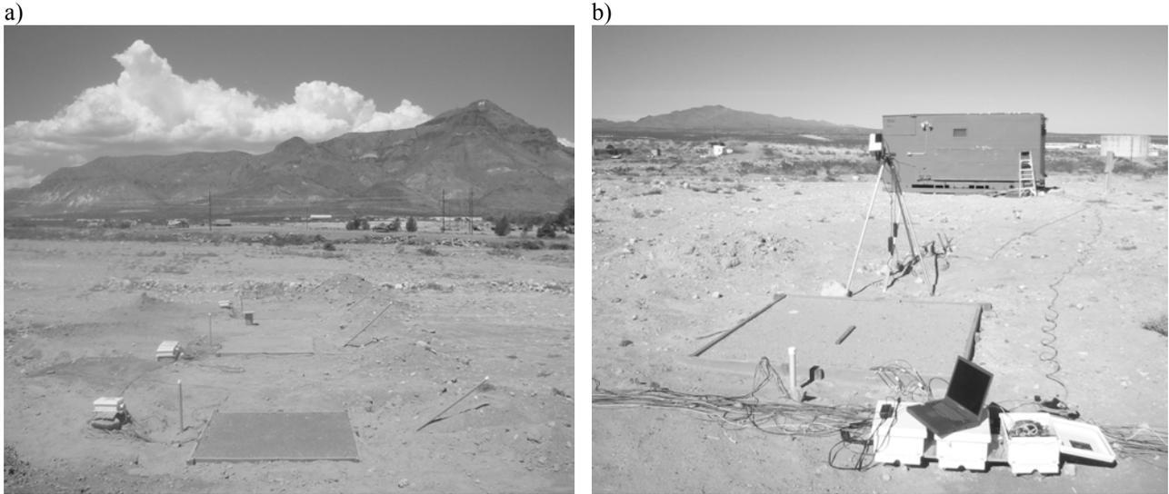
Fig. 1. a) The NMT outdoor land mine detection test facility at the foot of “M-mountain”. b) The setup in detail with datalogger and sensor control in the white boxes in the foreground and the field office in the background.
