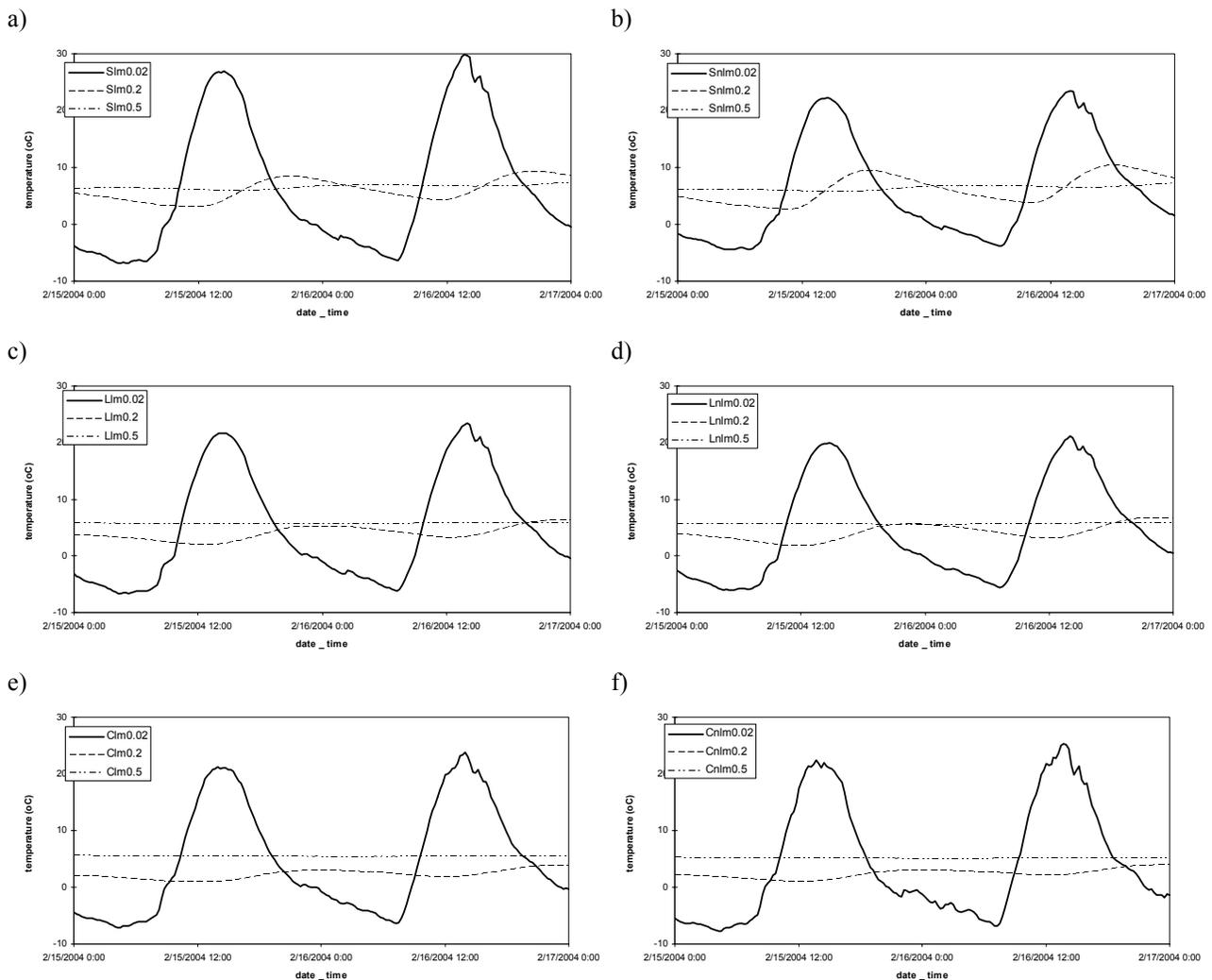
Fig. 7. Time series showing temperature distribution for different soils and at different depths. a) Sand soil, above and below land mines; b) homogeneous sand soil; c) Loam soil, above and below land mines; d) homogeneous loam soil; e) Clay soil, above and below land mines; f) homogeneous clay soil. The numbers in the legends refer to the depths of the temperature probes, 0.02, 0.2 and 0.5 meters.
