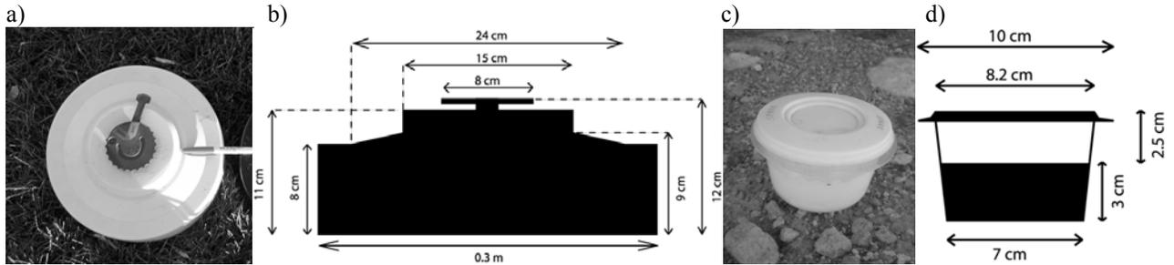
Fig. 3. Pictures and schematic diagrams with dimensions of buried land mines. Picture (a) and dimensions (b) of the NR26 simulant AT land mine. Picture (c) and dimensions (d) of NMT fabricated simulant AP land mine.
