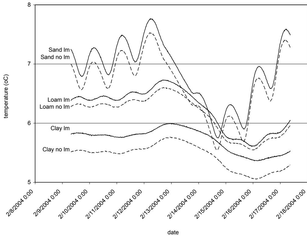
Fig. 8. Plot of soil temperatures for an eight-day period in February 2004 at 0.5 meters depth in three soil types. “lm” stands for a temperature measurement under an AT land mine simulant. “no lm” stands for a temperature measurement in homogeneous soil.
