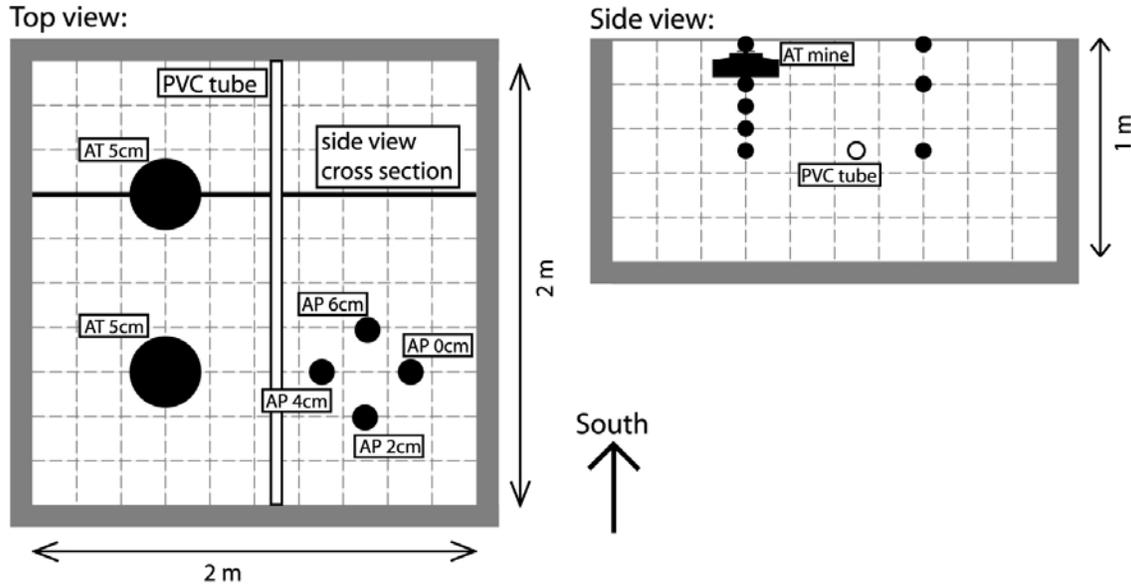
Fig. 2. Layout of the test plots at the NMT land mine detection test facility. In the side view, the open circle marks the location of the PVC tube. The black circles mark the locations of the temperature and soil moisture sensors.
