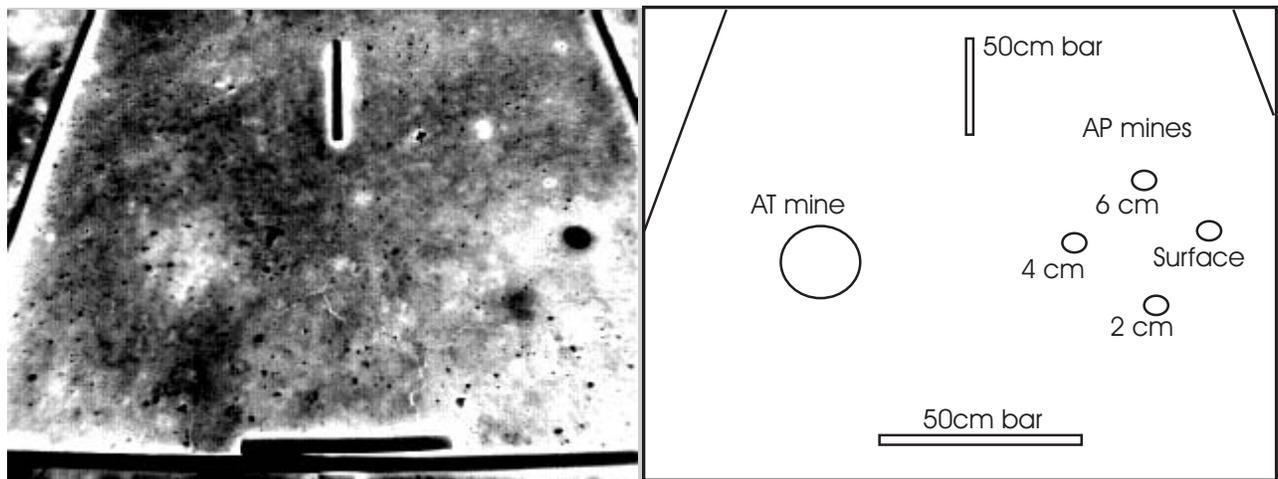
Fig. 9. Thermal infrared image of the loam test plot at 6:40 PM on January 28, 2004. The surface temperature differs 5.5 °C between the area above the AT mine simulant (warm) and the AP mine simulant at the surface (cold).
