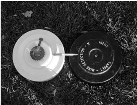
Figure 1: Surrogate antitank mines (30 cm diameter). The left mine surrogate was used in this study.
