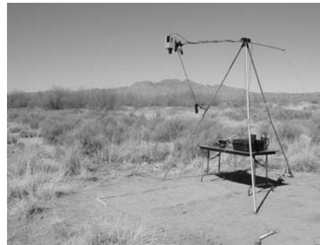
Figure 2: Infrared camera setup for thermal signature
