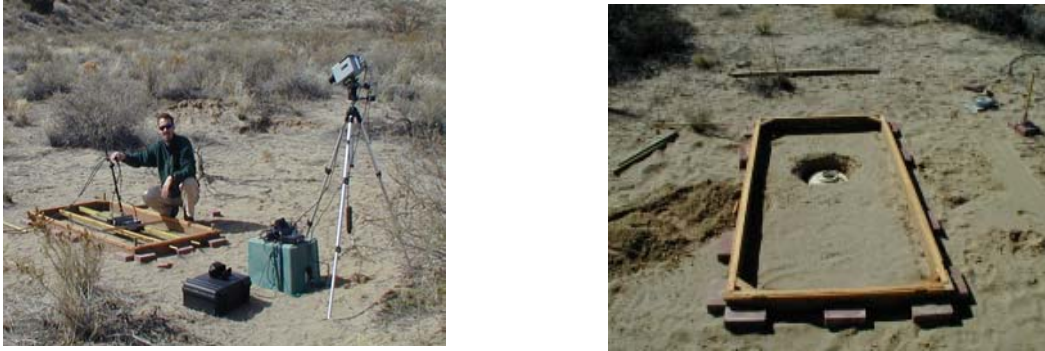
Figure 2: Field area with the ground penetration radar system at a frequency of 900 MHz and IR camera (A) and geometry of antitank landmine installation (B).
