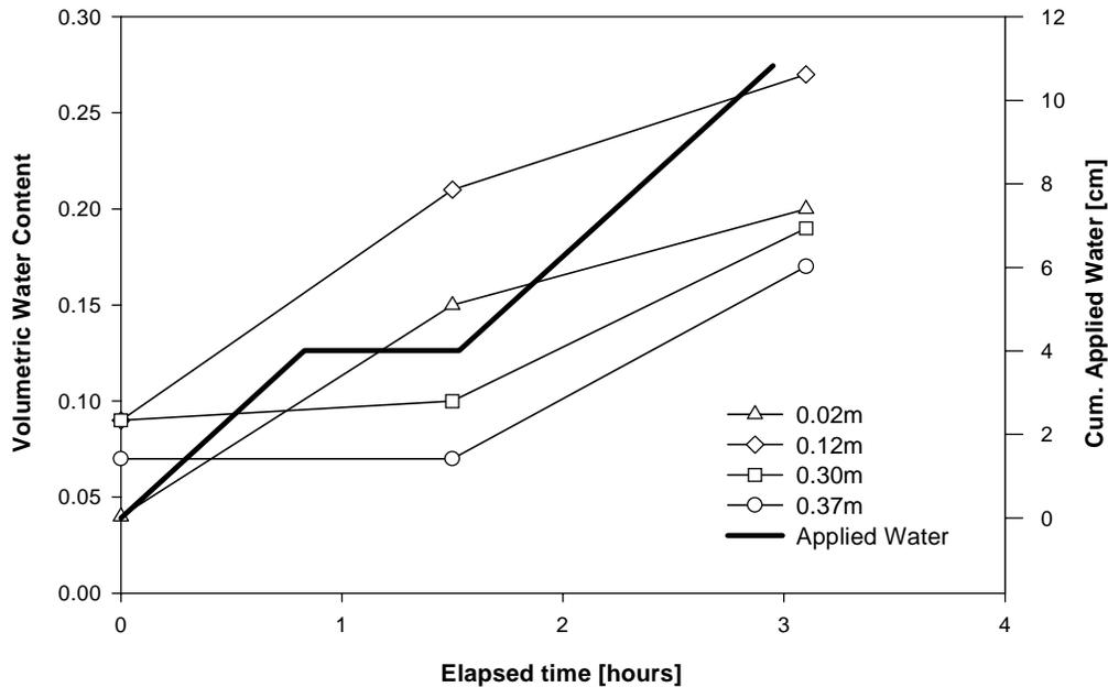
**Figure 4:** Measured soil water contents above and below the mine.
