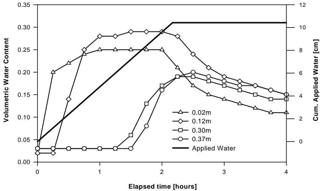
**Figure 3:** Hydrus-2D Simulation of water contents above and below the mine.
