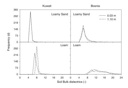
Figure 6: Frequency of dielectric constant close to the mine (r=0.03 m) and away from it (r=1.1 m).
