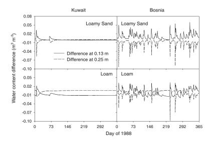
Figure 5: Water content at observation point x1 minus water content at observations point x3 (0.13 m) and water content at observation point x2 minus water content at observation point x4 (0.25 m).
