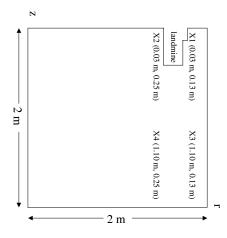
Figure 1: Layout for the simulation of water distributions around landmines with four observation points x1, x2, x3, x4.
