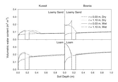
Figure 4: Soil water content versus depth at the center of the mine (r=0.03 m) and away from it (r=1.1 m) under dry conditions (day 215 in Kuwait and Bosnia) and wet conditions (day 10 in Kuwait and day 235 in Bosnia).
