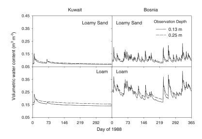
Figure 3: Soil water content changes during 1988 at observations points x3 (0.13 m) and x4 (0.25 m) in a Loam and Loamy Sand in Kuwait and Bosnia.
