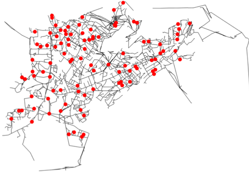
Figure 2.2: The network used for the simulation study. Injection locations are highlighted.
